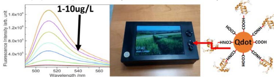
Scheme 1. Schematic representation of covalent coupling of biomimetic D1 peptide to carboxyl quantum dots by carbodiimide method and small fluorescence transducer device.
