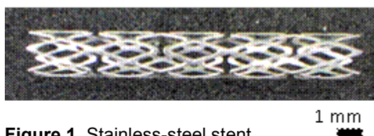
Figure 1. Stainless-steel stent fabricated using lithography and wet etching.
