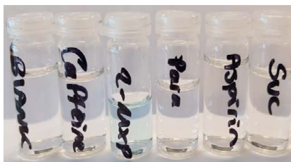
Figure 1. a) SDC test for 2-MXP. When incubating a dye-loaded 2-MXP MIP with two legal pharmacological compounds or two common adulterants, no color change is observed. Incubation with 2-MXP leads to dye displacement and coloring of the filtrate b) schematic illustration of the multi drug sensing device.
