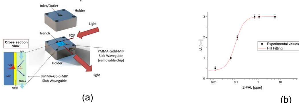
Figure 1. (a) Chemical SPR sensor outline. (b) Resonance wavelength variation (with respect to blank 0 ppm) versus 2-FAL concentrations, in semi-logarithmic axes, for SPR-Slab-MIP, with the Hill fitting of data.
